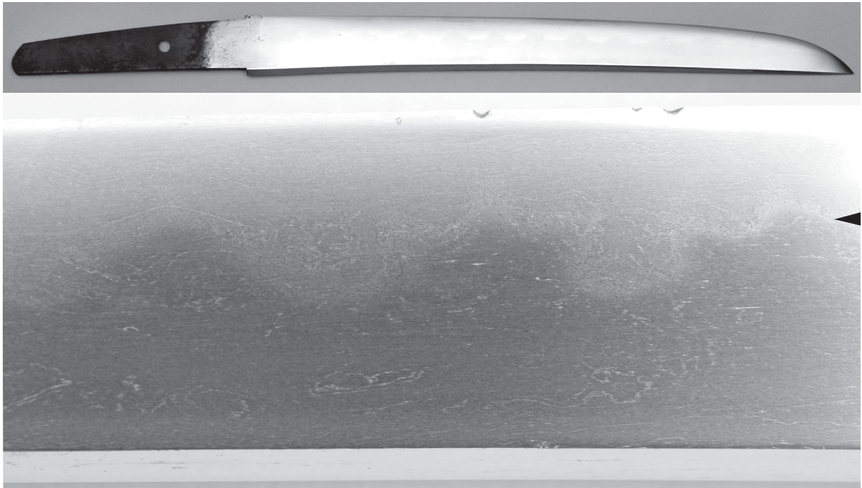
Nioi appearing as a misty line along the hamon in a 17th Century Japanese tanto (dagger) blade. As the hamon is a boundary formed at the time of quenching, the term 'temper line' is a misnomer.
