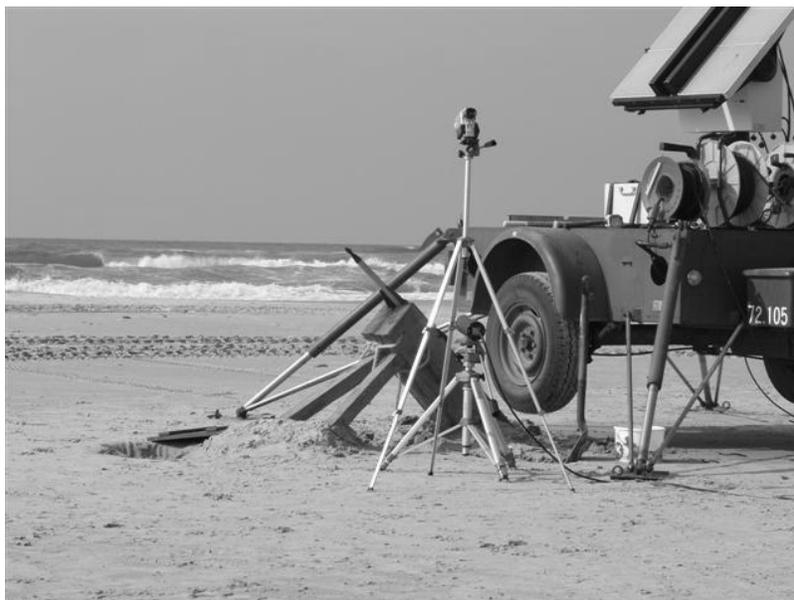
Fig. 2 The Loshult gun loaded with the replica of an Eltz arrow ready to fire. In front on the right the head for measuring muzzle velocity and, higher a video camera can be seen. The radar antenna for measuring and recording the trajectory of the arrow can be seen in the upper right hand corner. Photograph by the author
