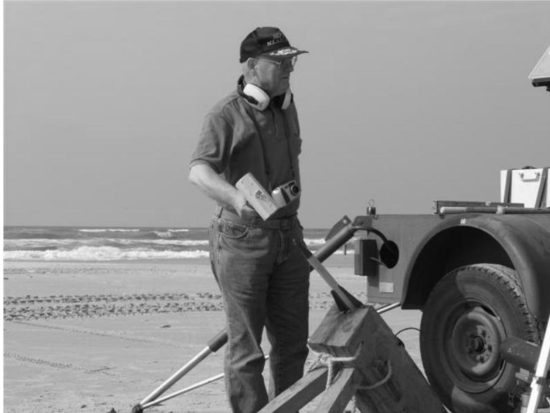
Fig. 3 The author loading the Loshult gun at the shooting range at Oxbøl. The arrow is seated with a wooden mallet. The fuse cord can be seen between gun and tyre. Photograph by Bob Smith
