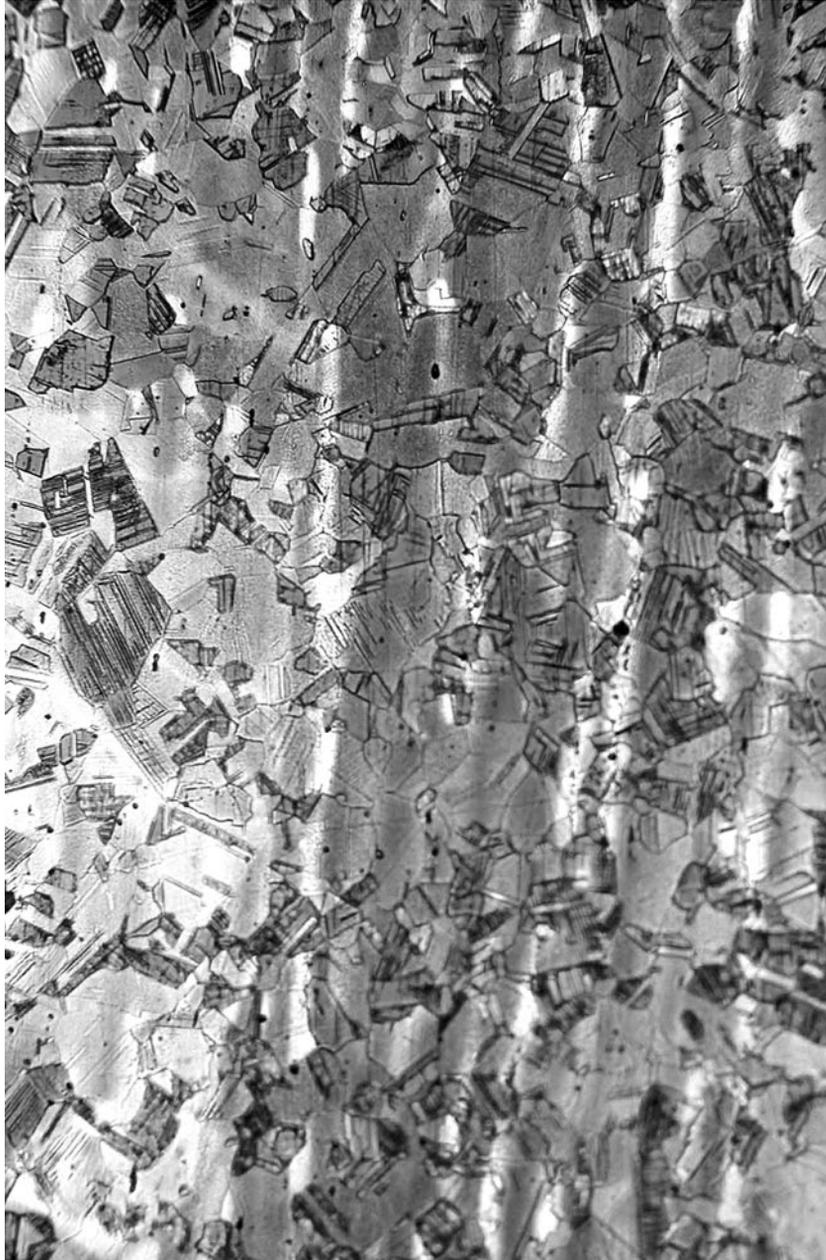
Fig. 17. Micrograph for the small button (WK.A150-9) at a magnification of 200 $\times$ , for a v-shaped section cut from the rim.
