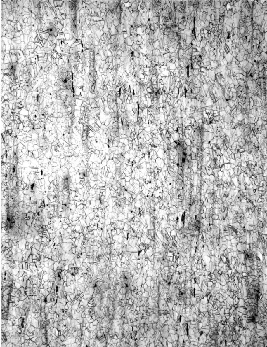
Fig. 11. Micrograph for the vessel (WK.B196-5) at a magnification of 200 $\times$ , for a v-shaped section cut from the rim.
